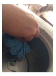
USE A CLEAN CLOTH TO CLEAN UP ALL THE WATER IN COLD TANK, CLEAN THE SIDES OF TANK MAY BE CALCUIM BUILD UP HERE...
